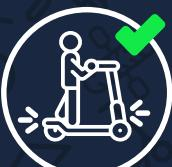
A personal light electric vehicle must be equipped with a white light at the front and a red light at the rear and a yellow, red or white reflector or light on the sides. § 87 (1(2))
